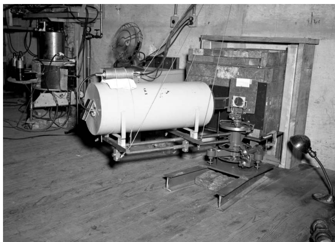
Figure 10 Wollan's crystal spectrometer at the graphite reactor in Oak Ridge in 1946.
